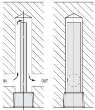
The position of the baffle board in the direction of rotation should be wrapped with sealing tape or the like to adjust the tightening. · Processing example of baffle boards
