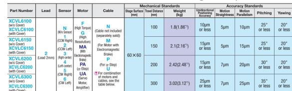
1. When the "With Cover" ootion is selected T. When the Motor Ootion M. P. U and is unavailable for Ootion M The value differs depending on the type of motor. The above values are for stages incorporating Motor F (High Torque).
