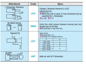
Features: Straight Slot Pins for Inspection Jigs. Handle lengths are selectable. For compatible bushings, see P.1841~P.1844.
