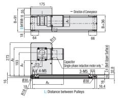
Motor mounting position specifications for TM5
